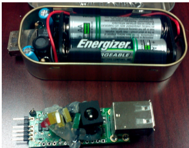
Figure 4. An extremely compact USB duplicator
